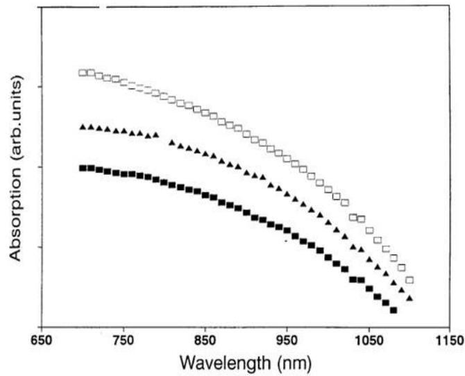
Fig. 4 UV-Vis - NIR spectra of Ge<sub>20</sub>Bi<sub>x</sub>Se<sub>80-x</sub> glasses.
