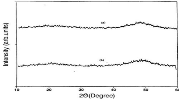
Fig. 1 X- ray diffraction pattern of (a)  $Ge_{20}Bi_{10}Se_{70}$  and (b)  $Ge_{20}Bi_{10}Se_{70}$  glasses.
