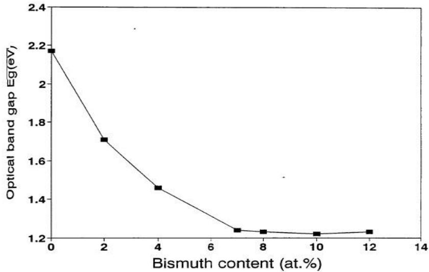
Fig. 5 Variation of the optical band gap  $E_g$  with average coordination number  $Z$  for the  $Ge_{20}Bi_xSe_{80-x}$  glasses using UV-Vis-NIR absorption technique.
