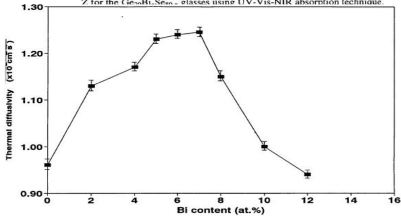
Fig. 6 Variation of thermal diffusivity  $\alpha$  with average coordination number  $Z$  for  $Ge_{20}Bi_xSe_{80-x}$  glasses.
