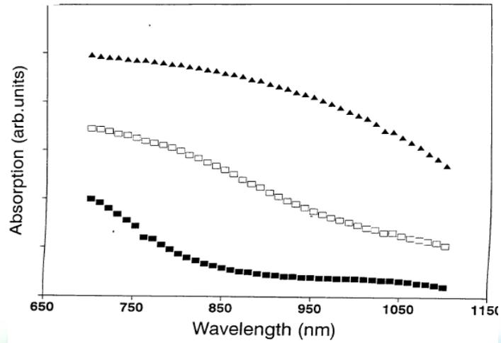
Fig. 3 UV-Vis - NIR spectra of Ge<sub>20</sub>Bi<sub>x</sub>Se<sub>80-x</sub> glasses.
